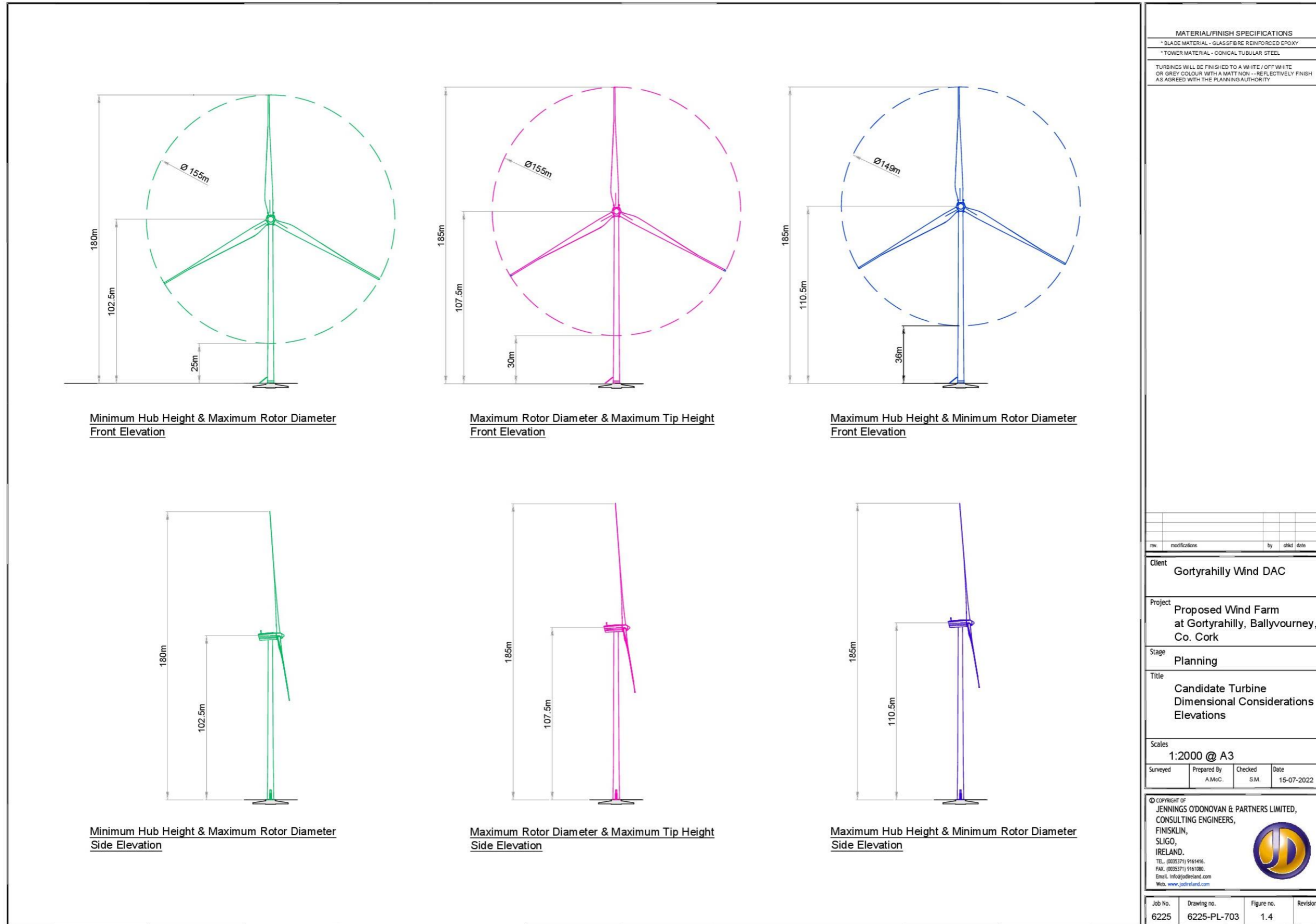
Figure 1.1: Candidate Turbine Dimensional Considerations Elevations
